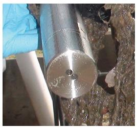
Ultrasonic cleaning technology is capable of preventing biofouling of the sensors in very harsh conditions saving time and money on sensor maintenance.
